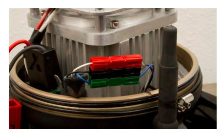
Plug freediving electronics into 2 point connector for freediving remote operation.
